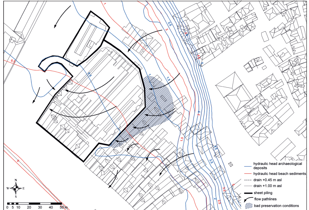
Figure 10. Steady-state simulated phreatic level within the archaeological deposits and the hydraulic (pressure) head in the beach sediments below the archaeological deposits. Arrows indicate general horizontal flow direction.
