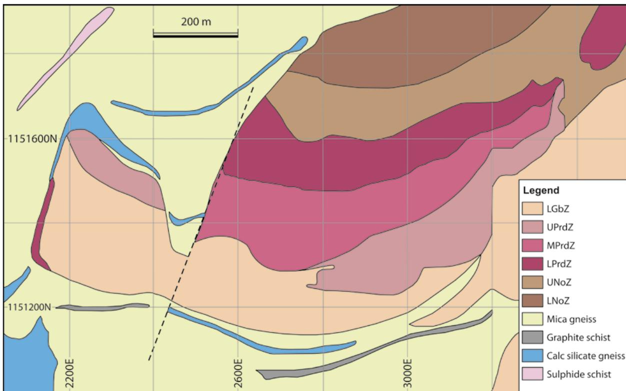
**Figure 10: Geological map of the Bruvann area** (Lamberg 2005, modified after Boyd & Mathiesen 1979 and Karppanen et al. 1999) (Gb= gabbro, Prd= peridotite, No= norite)
