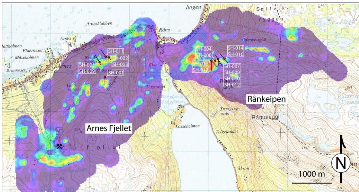
**Figure 6: Results from SkyTEM survey and location of holes drilled by Scandinavian Highlands in 2006 - 2007**
