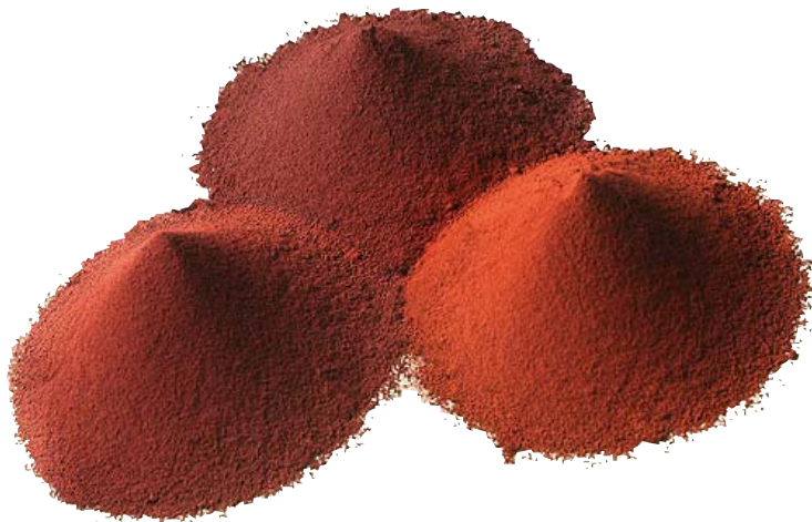
Three different types of pigment consisting of the iron oxide, hematite, produced by Rana Gruber. The pigments are used in concrete, paint, lacquer, cosmetics and other applications. Photo: Rana Gruber AS
