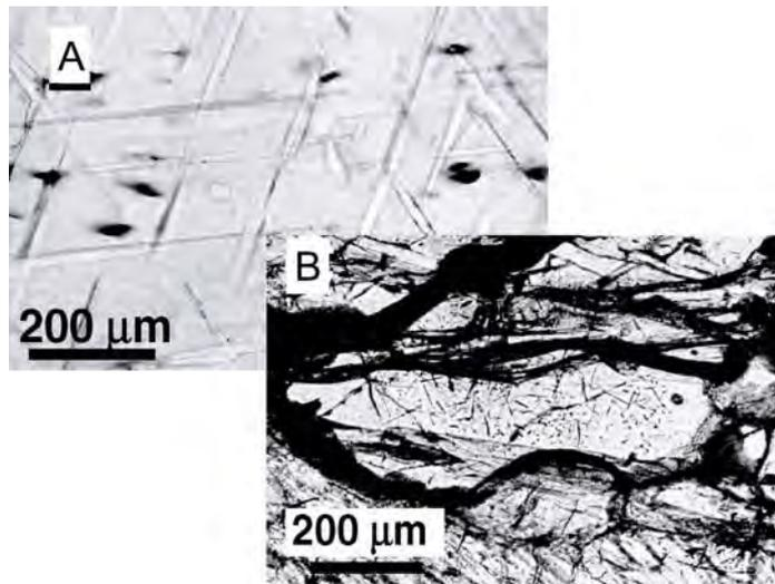
**Fig. 7.3** Optical micrographs illustrating pyroxene exsolution from garnet. A) Garnetite; Otrøy garnet peridotite (M2). B) Garnet websterite; Bardane (M3). Note: scale-difference, both images were taken with the same magnification.
