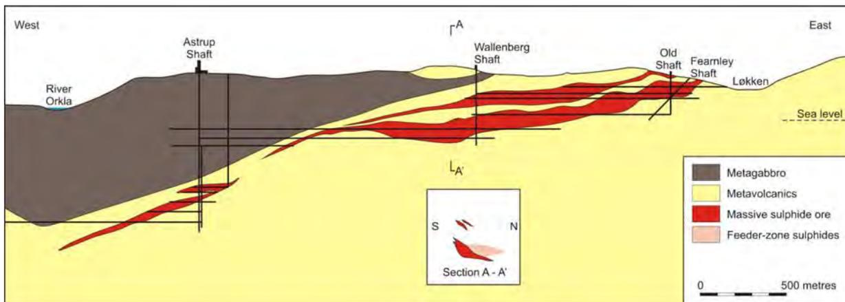
Fig. 6.6. Vertical longitudinal section and cross-section of the Løkken massive sulphide deposit. Modified from Grenne et al. 1980.
