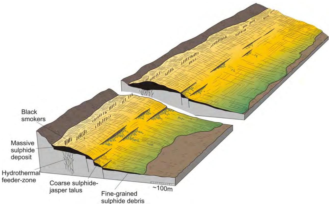
Fig. 6.7. Pre-deformation reconstruction of the Løkken orebody during deposition from hydrothermal vents (including 'black smokers') along fault scarps on the sea floor.
