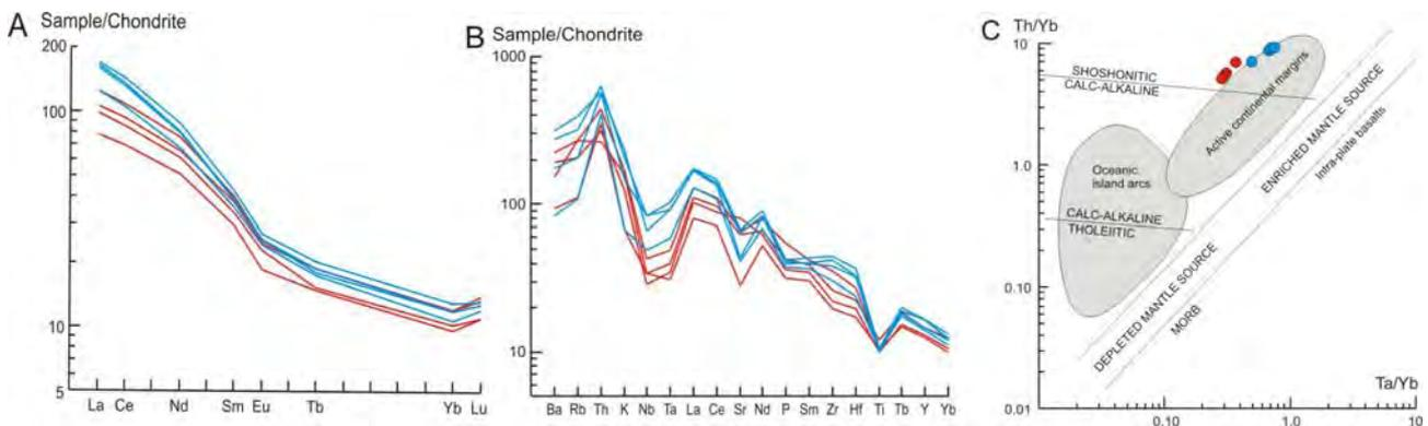
Fig. 6.2. Geochemistry of the Hølonde Porphyrites. A) Chondrite-normalised REE patterns; B) chondrite-normalised trace element patterns; C) Th/Yb vs. Ta/Yb discrimination diagram. Modified from Grenne & Roberts (1998). The blue and red colours represent two slightly different magma series.
