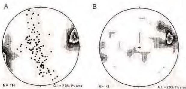
Summary of structural data for the Ullaholmen exposure. A. Contours of lineations and poles to foliation. B. Contours of fold axes.
