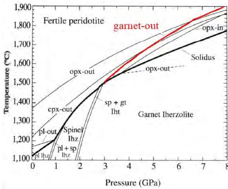
**Fig. 7.9** Generalised phase diagram for fertile peridotitic mantle, based on experimental data for dry peridotite melting (Takahashi 1990; Walter 2003).
