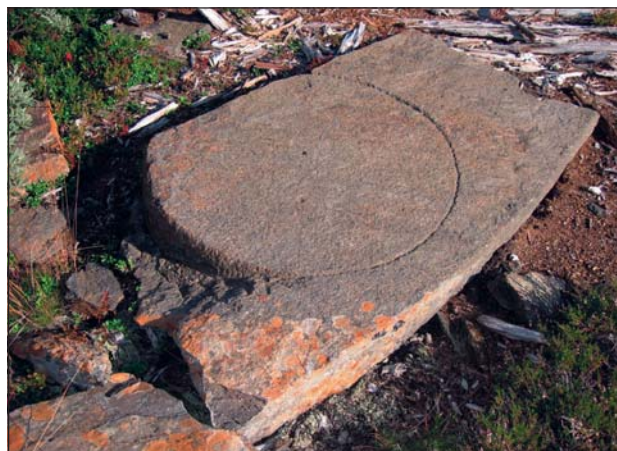
Figure 27. Marks after a compass used to outline a planned millstone in Selbu. Carving of the millstone side was finished almost through the slab before it continued along the rest of the compass markings.
