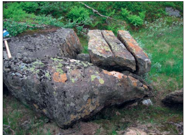
Figure 22. Primitive extraction of millstone slabs from the Brennrya area in the Nordfjellet quarry landscape, Selbu. Three slabs are variably loosened from a small cliff by cutting grooves along the primary cleavage.
