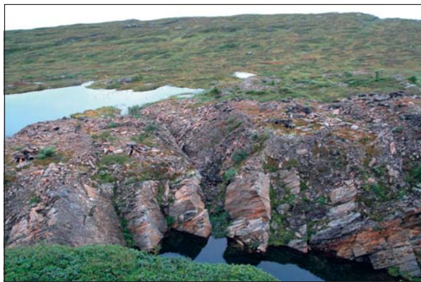
Figure 25. Westerly view of the large Raudhammeren quarry, from the latest period of quarrying in Selbu. Note the cross fractures that were appropriately spaced for production of large blocks. An open adit enters the quarry from near the lake. On top of the irregular waste heaps and working areas on the quarry margin, one can see three remains of timber capstans used to lift waste and blocks. An area with much older, pre-powder quarries is seen in the background to the right of the lake.
