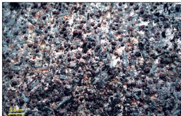
Figure 7. Close-up of weathered surface of garnet-kyanite-muscovite schist (coarse-grained variety) from the Hyllestad millstone quarries.
