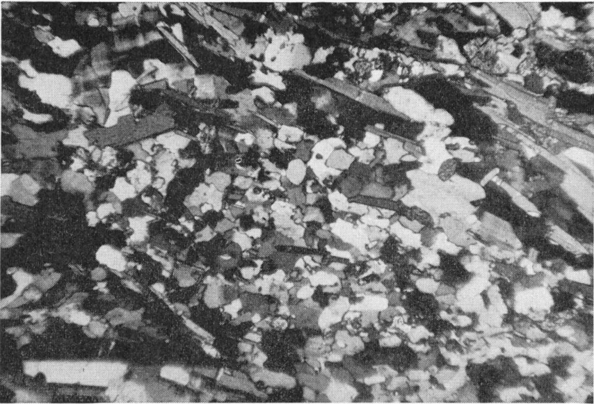
Fig. 11. Fine grained granite gneiss within mica schists, Sitasjavrrre, Tysfjord area. The minerals are microcline, plagioclase, quartz, epidote and biotite (+n., 35x).
