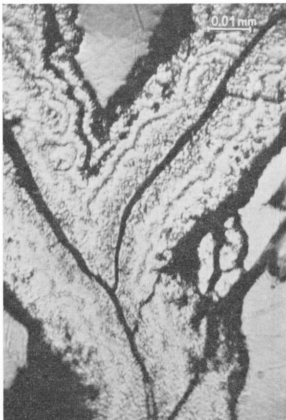
Fig. 15. Secondary pyrite along cracks in pyrrhotite.
