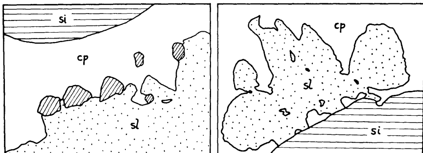
Fig. 44. Drawings from photomicrographs showing chalcopyrite-sphalerite relationships. a) Sphalerite (sl) "front" replacing chalcopyrite (cp) but not attacking grains of pyrrhotite (shaded). Skaide. X 130. b) Irregular replacement patch of sphalerite (sl) in chalcopyrite (cp). Skaide X 300.
