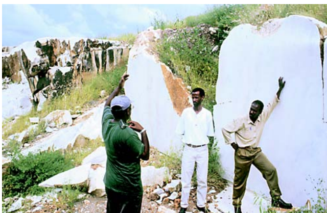
Fig. 2. Prospect of white calcite marble in the Gogne area, SW Eritrea. Diamond wire has been used for vertical cutting.
