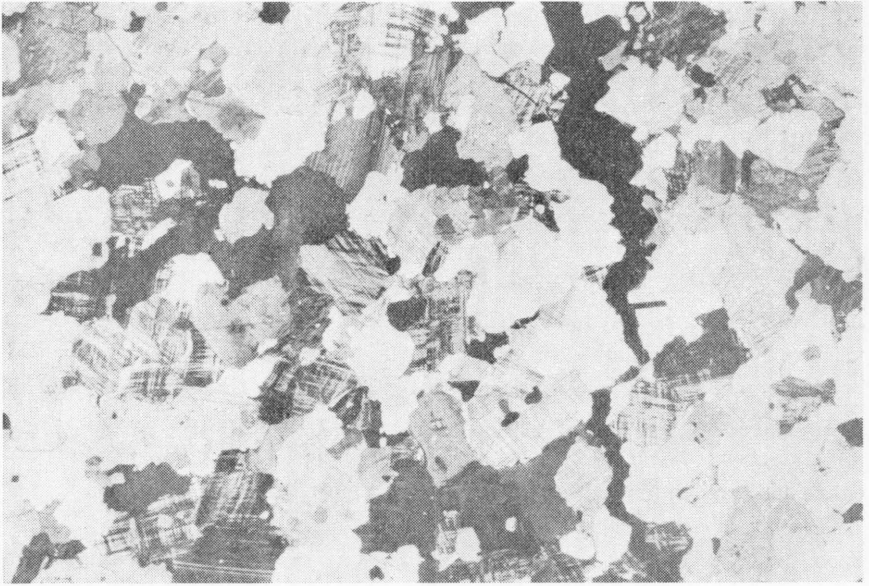
Fig. 32a. Photomicrograph of Fyresdal granite: Specimen taken from the border of granite. Crossed nicols, X 33,5.
