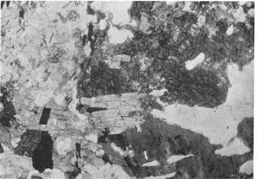
Photo No. 3. Amphibolite; hornblende replaced by biotite, quartz and epidote, which also replaces plagioclase, ( \times 35 , plane polarised light).
