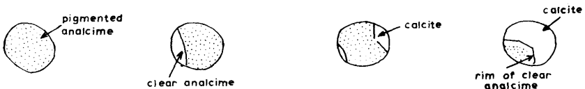
Fig. 3. Various globular ocelli consisting of analcime and calcite. The ocelli are about 2 mm in diameter.
