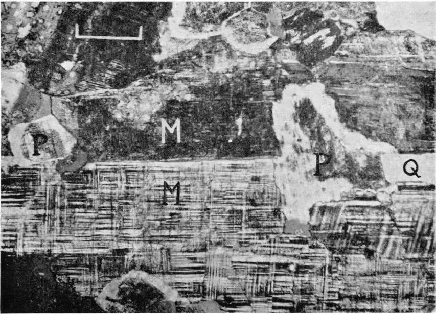
Fig. 1. Plagioclase (P) and Quartz (Q) inclusions in Microcline (M). The white line is 1 mm long. Crossed polars. Plagioklas og Kvarts inneslutninger i Mikroklin.
