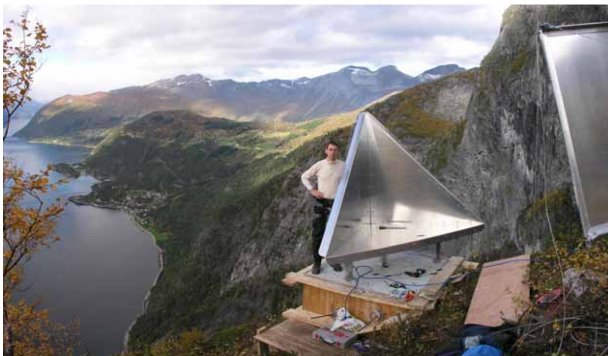
Figure 17. Artificial corner reflector installed near Tafjord, in Norway. The reflector is constructed of 10mm thick aluminum.
