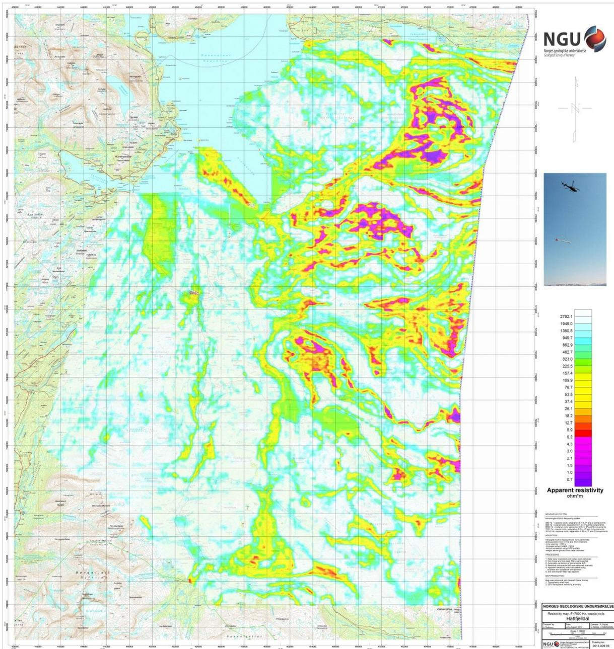
Figure 10: Apparent resistivity. Frequency 7000 Hz, Coaxial coils
