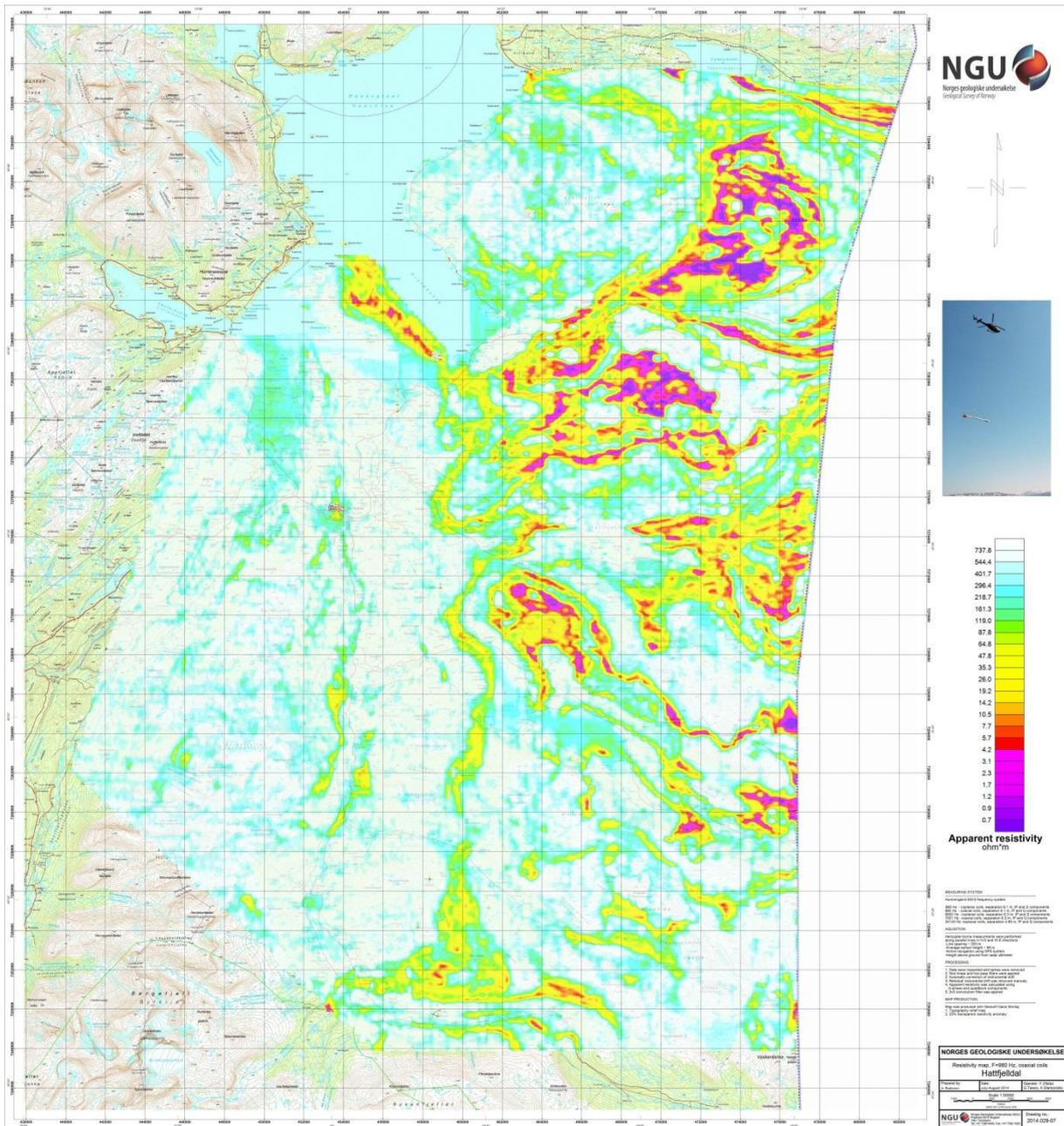
Figure 11: Apparent resistivity. Frequency 7000 Hz, Coaxial coils
