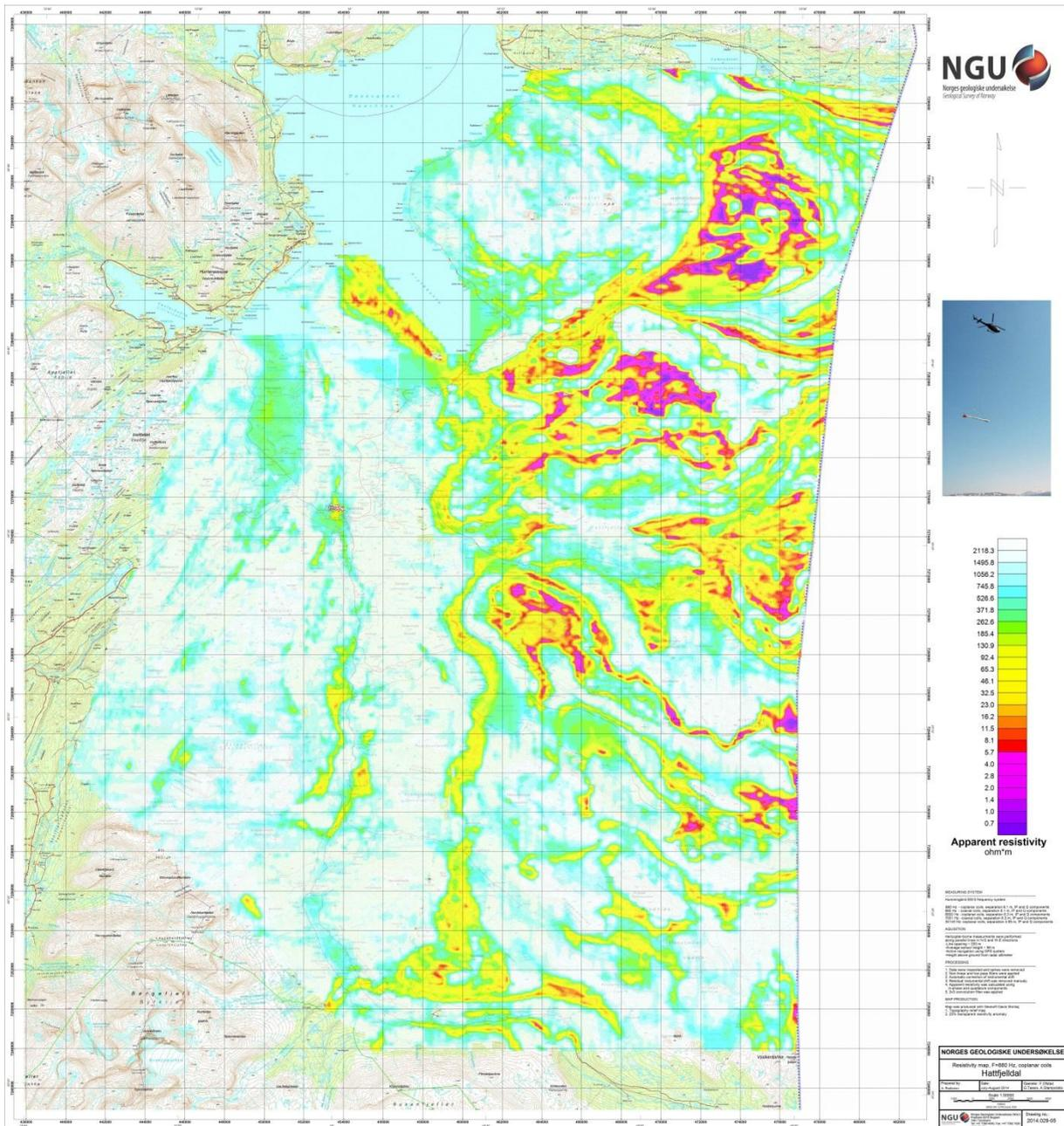
Figure 9: Apparent resistivity. Frequency 880 Hz, coplanar coils
