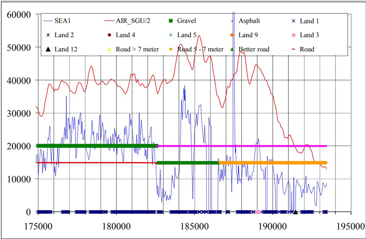
Figure 5.3. ESD for  $^{137}\text{Cs}$  along the last part of the definitive route: CGS system SEA1 compared to the AGS measurements by SGU (divided by 2).
