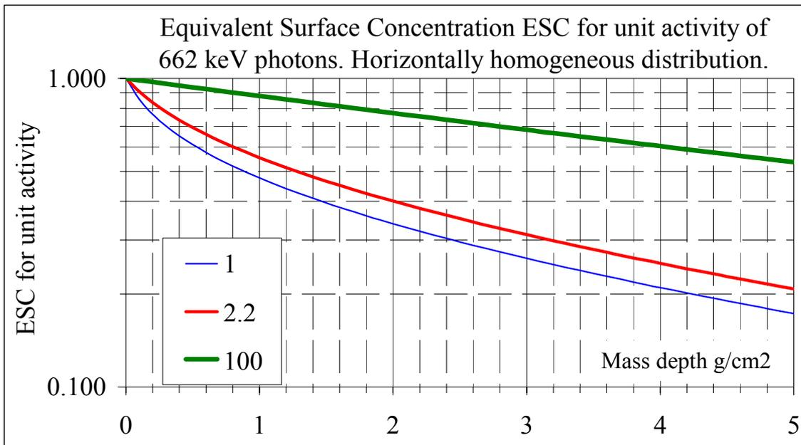
Figure 3.2. ESC for unit activity of  $^{137}\text{Cs}$ . Mass depth 0-5  $\text{g}/\text{cm}^2$ .
