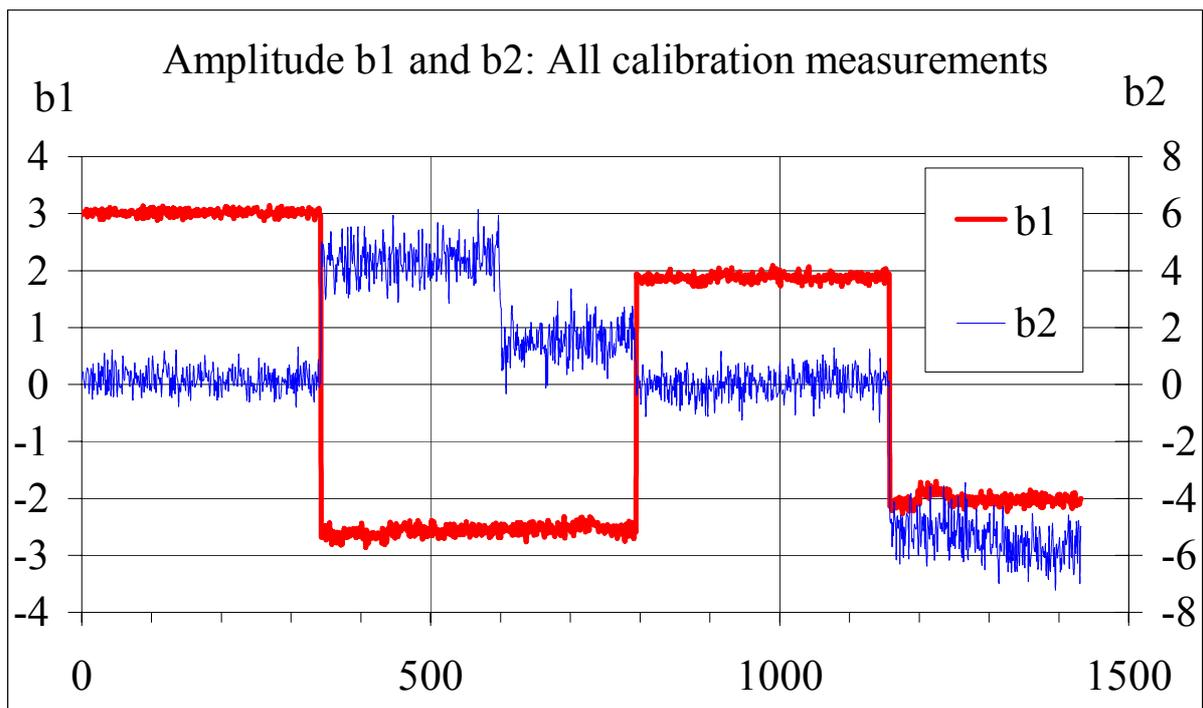
Figure 4.5. Amounts of spectral component S1 and S2 contained in the measurements. NASVD procession of all reference measurements. Plateaux from left to right (b1): Älvkarleö, Harnäs, Regementsparken and Utvalsnäs.
