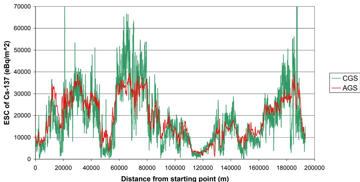
Figure 5.5. ESC for  $^{137}\text{Cs}$  along the whole definitive route: AGS and CGS (median car) both normalised to system DKA1.
