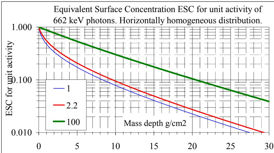
Figure 3.1. ESC for unit activity for  $^{137}\text{Cs}$ . Mass depth 0-30  $\text{g}/\text{cm}^2$ .
