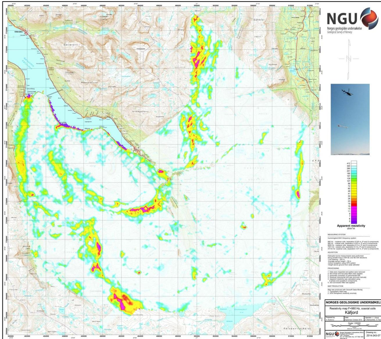
Figure 11: Apparent resistivity. Frequency 980 Hz, Coaxial coils
