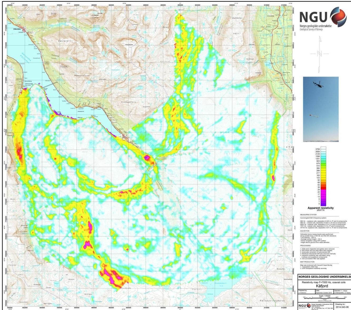
Figure 10: Apparent resistivity. Frequency 7000 Hz, Coaxial coils
