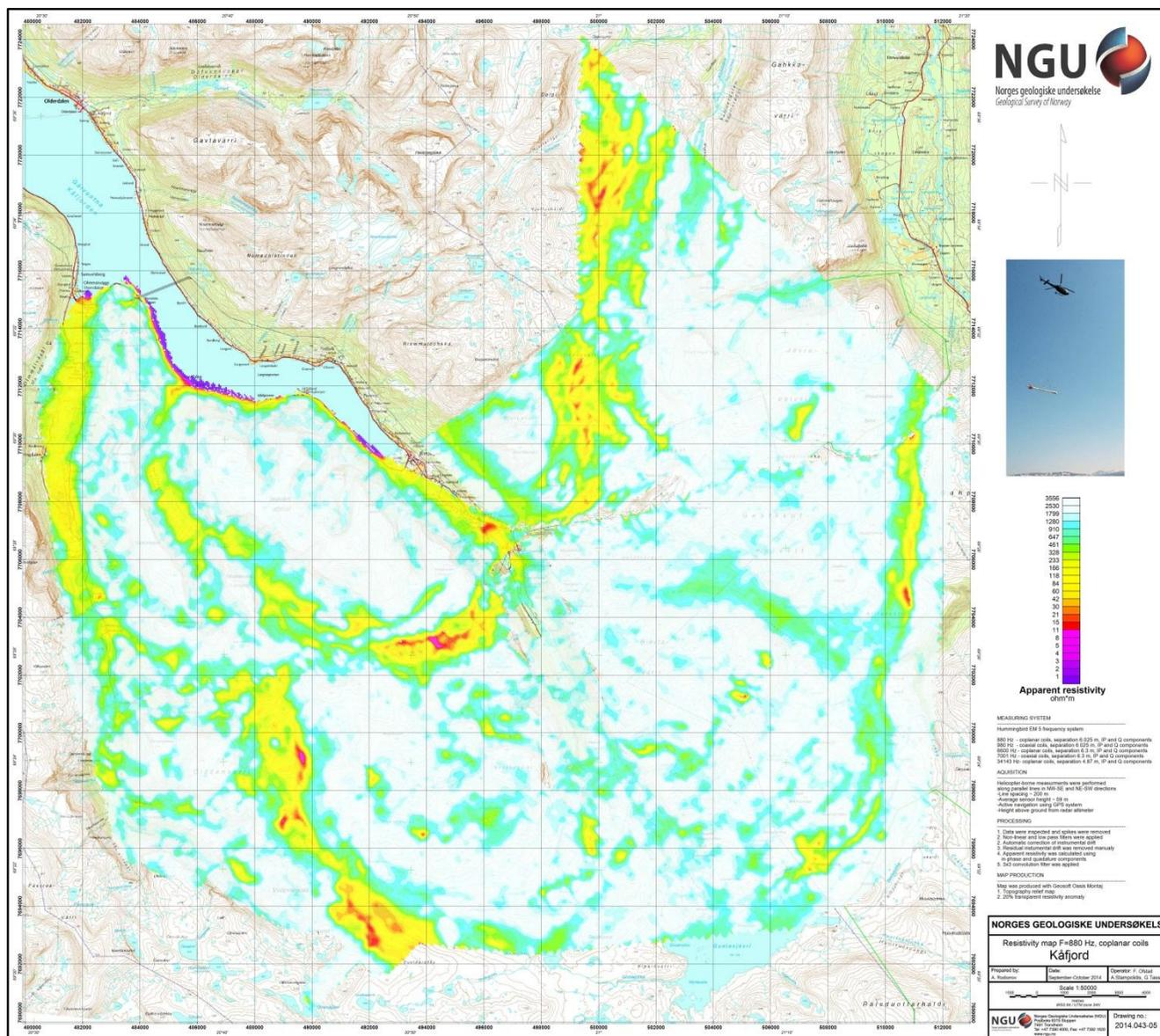
Figure 9: Apparent resistivity. Frequency 880 Hz, coplanar coils
