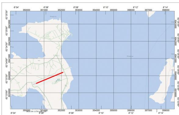
To determine coefficients of calibration for the laser and radar altimeter, steps are flown at 5 different heights, from 40m to 180m and over the Alta airport strip in order to have a surface as flat as possible for the calibration. In order to minimize errors, each step is 2 km long.
