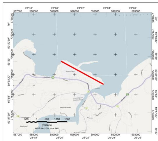
To determine coefficients of calibration for the laser and radar altimeter, steps are flown at 5 different heights, from 40m to 180m and over the Alta airport strip in order to have a surface as flat as possible for the calibration. In order to minimize errors, each step is 2 km long.
