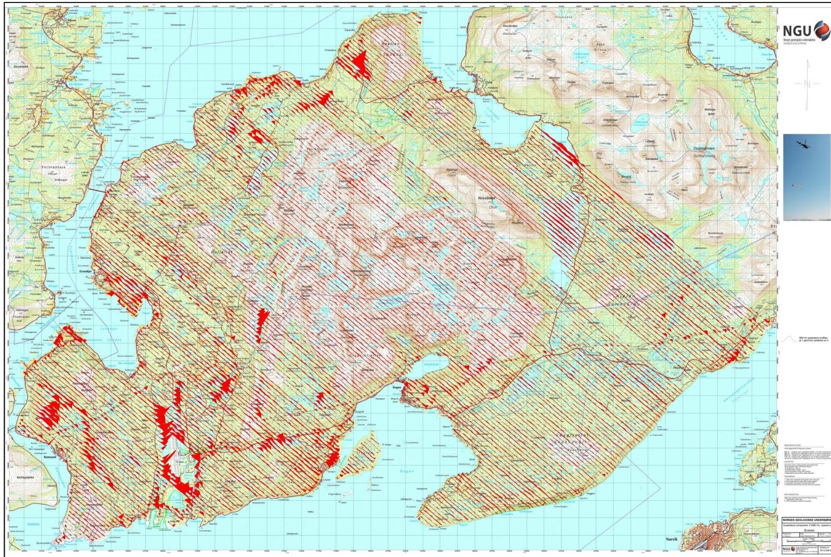
Figure 11: Quadrature component. Frequency 980 Hz, Coaxial coils
