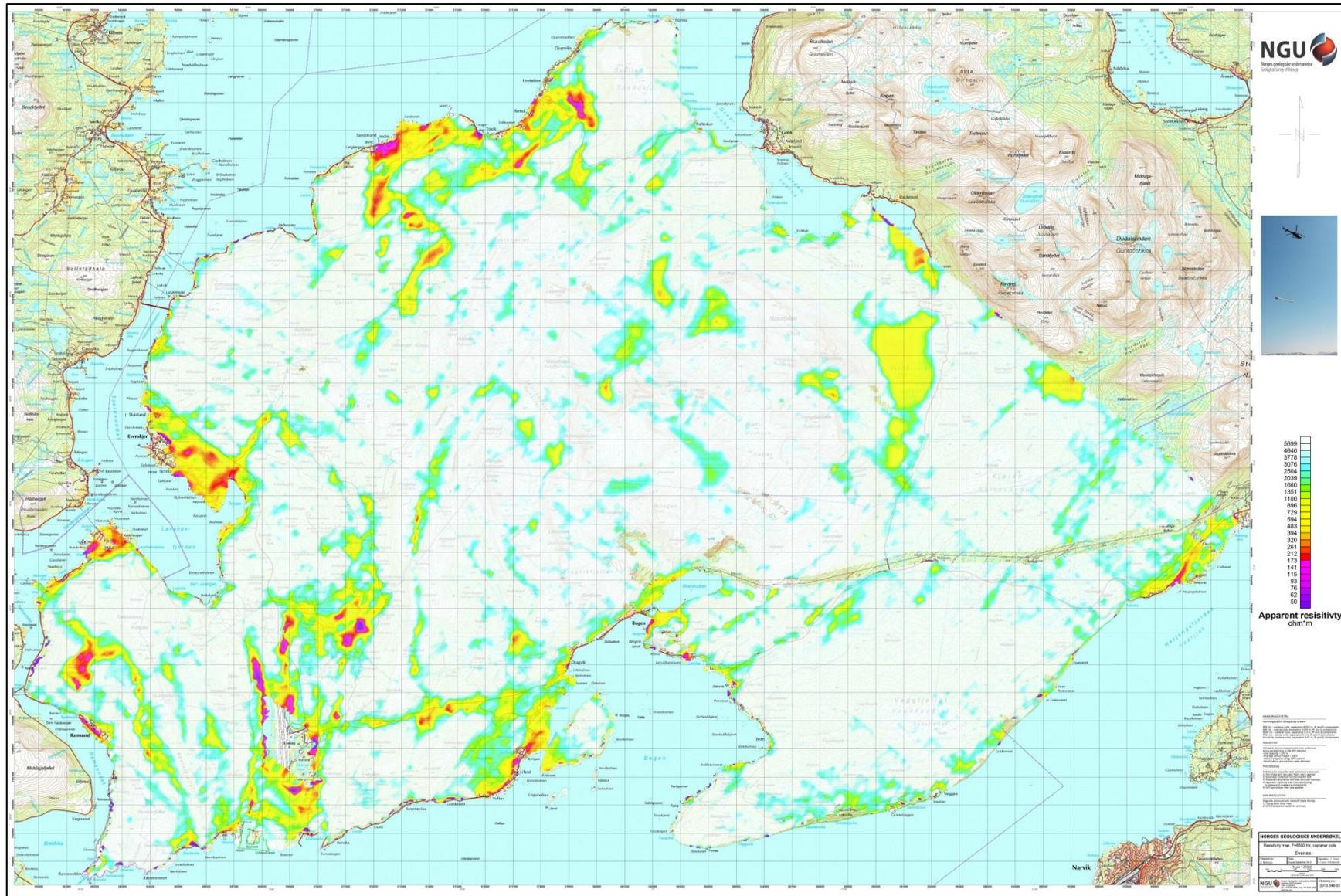
Figure 8: Apparent resistivity. Frequency 6600 Hz, Coplanar coils
