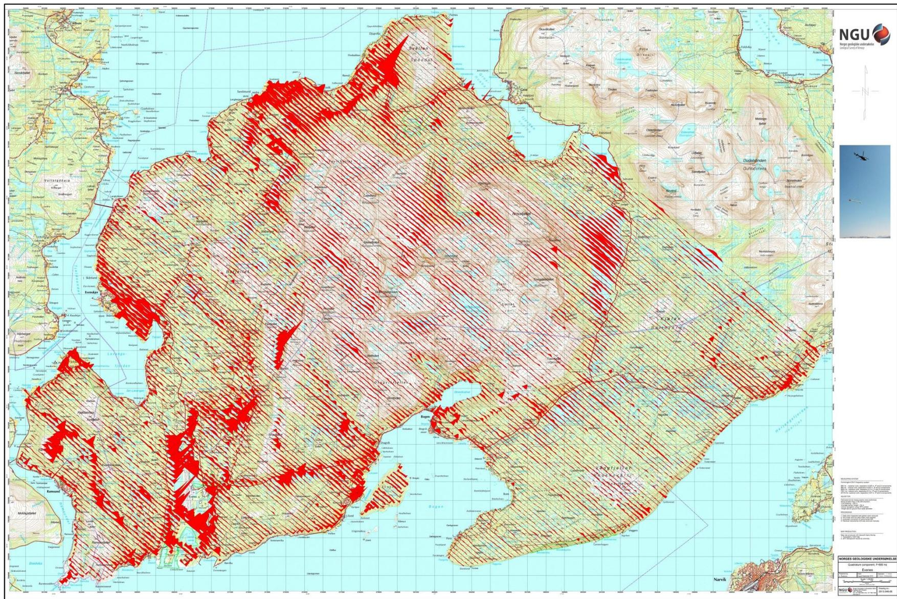
Figure 9: Quadrature component. Frequency 880 Hz, coplanar coils
