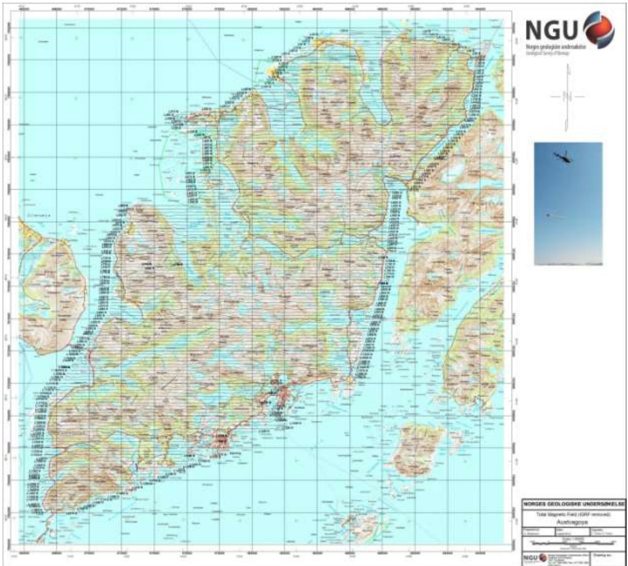
Figure 3: Austvågøya survey area with flight path
