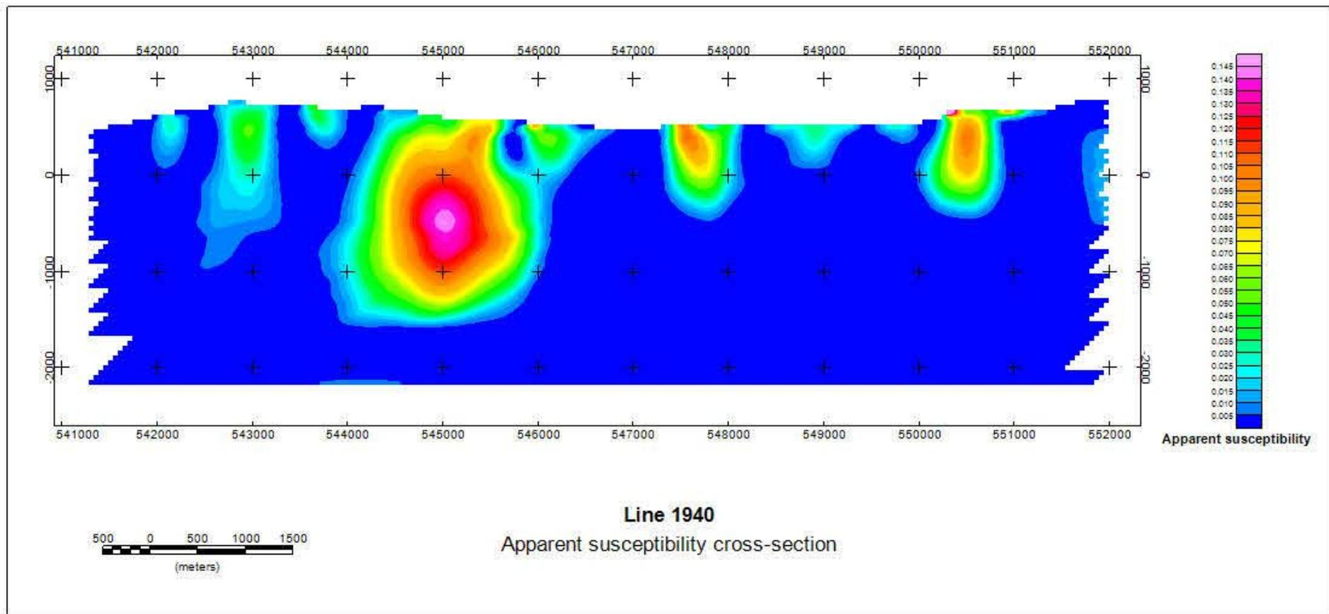
Figure 2: Apparent susceptibility cross-section, line 1940 (see Figure 4).
