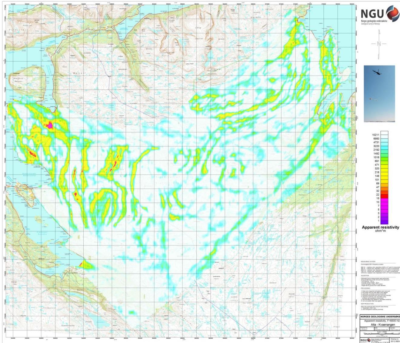
Figure 8: Apparent resistivity. Frequency 6600 Hz, Coplanar coils
