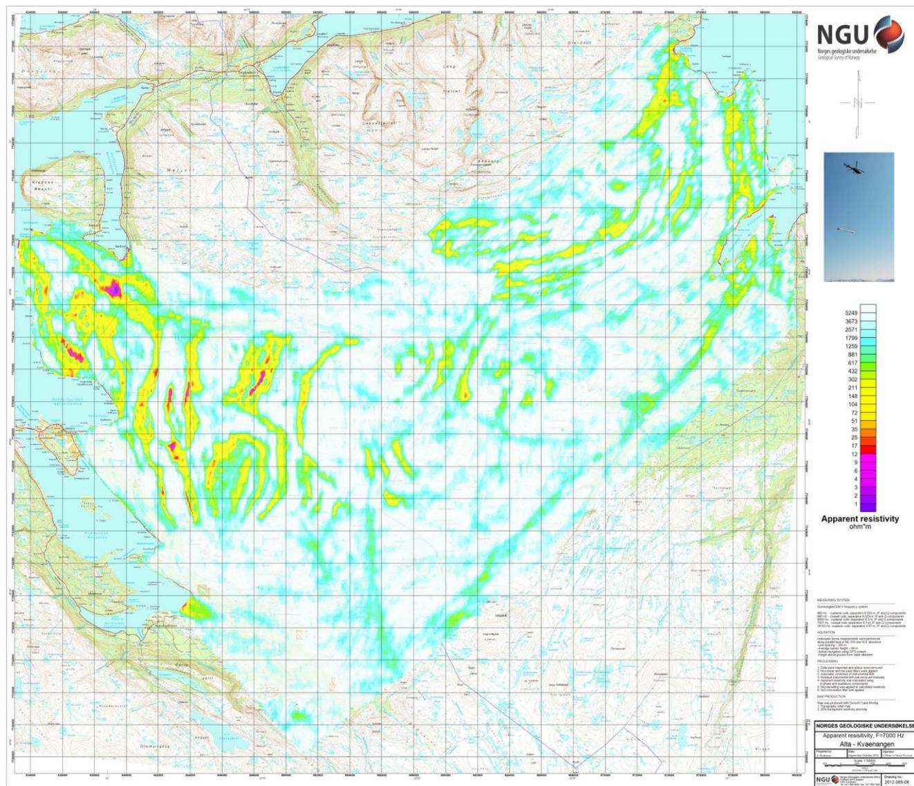
Figure 10: Apparent resistivity. Frequency 7000 Hz, Coaxial coils
