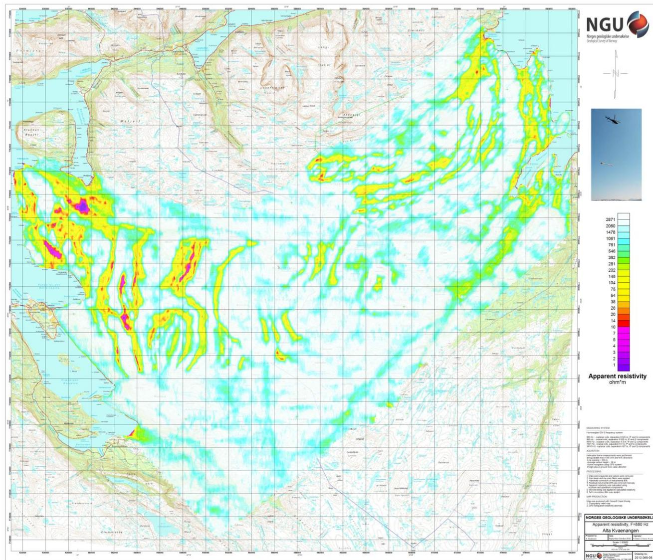
Figure 9: Apparent resistivity. Frequency 880 Hz, Coplanar coils
